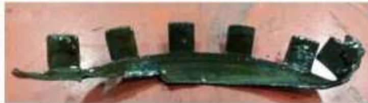
Image 3 of the failed tab washer found in the bearing cap from the 1 st Intermediate shaft.
